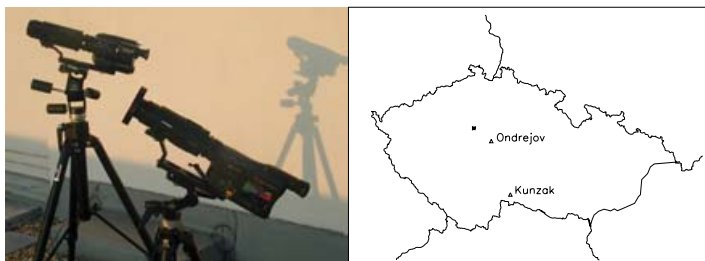
Figure 1. Left: Image intensifiers Dedal 41 mounted in front of videocameras (S-VHS Panasonic); right: the map of the Czech Republic — the positions of our stations are marked (Prague is also shown).
