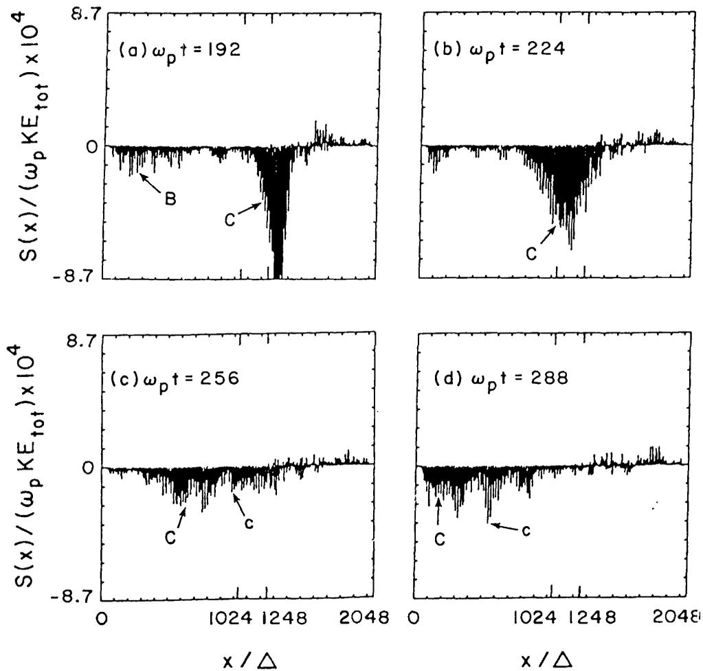
Fig. 2: Snapshots of the Poynting flux  $S(x)$  at four different times depicting the absorption of pulse C and a reemission event (pulse c). The absorbing plasma lies to the right of  $x/\Delta = 1248$ .
