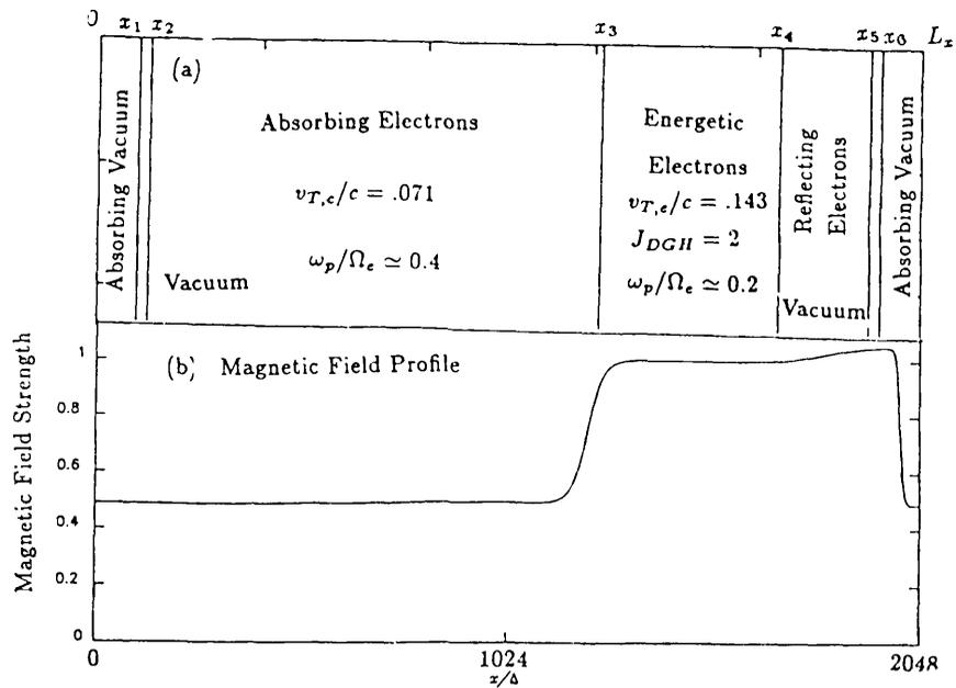
Fig. 1: The simulation model and the magnetic field profile. The magnetic field is perpendicular to the  $x$ -axis. The thermal velocity ( $v_T$ ) and ratio of plasma frequency to gyrofrequency ( $\omega_p/\Omega_e$ ) for the energetic and absorbing electron populations are shown.
