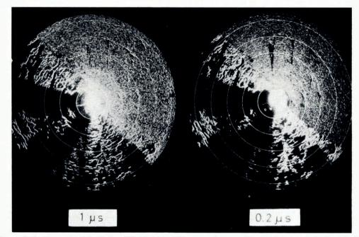
Fig. 1. Radar images observed with two different pulse widths, 0.2 and 1.0 µs. Coverage is 10 nautical miles (18.5 km).
