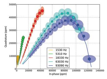
**Fig. 4.** Data from calibration site 1 (Table 2) with applied calibration coefficients. The instrument was lifted from zero (large dots) to  $2\,\mathrm{m}$  (smaller dots) over  $0.53\,\mathrm{m}$  thick sea ice with a conductivity of  $80\,\mathrm{mS\,m^{-1}}$ . The semi-axes of the ellipses indicate the in-phase and quadrature uncertainties. The forward models (solid curves) for  $0{\text -}3\,\mathrm{m}$  are shown for the different frequencies.
