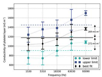
**Fig. 8.** Bulk platelet-layer conductivities. The results obtained at the different sites are averaged and shown for the individual frequencies. The conductivities and the corresponding standard deviations are shown for the best fit, and the lower and upper limit of uncertainties.
