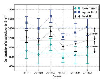
**Fig. 7.** Bulk platelet-layer conductivities. The results obtained using different frequencies are averaged and shown for the individual sites. The conductivities and the corresponding standard deviations are shown for the best fit, and the lower and upper limit of uncertainties. Dataset date format is day-month of 2012.
