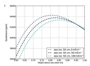
**Fig. 3.** Raw EM data  $(63\,030\,\text{Hz})$  for all Weddell Sea datasets. (a) Inphase, (b) quadrature and (c) enlargement of box in (b). The forward models (blue dashed curves) were calculated by assuming a homogeneous half-space of  $2700\,\text{mS}\,\text{m}^{-1}$  and resistive sea ice  $(0\,\text{mS}\,\text{m}^{-1})$ . Two additional forward models with increasing sea-ice conductivities  $(50\,\text{and}\,100\,\text{mS}\,\text{m}^{-1})$  are shown in (c).
