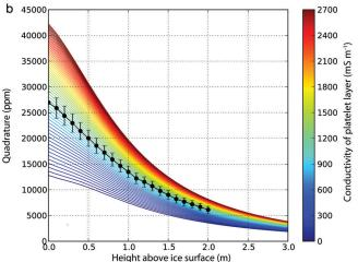
**Fig. 5.** Corrected dataset and corresponding uncertainties for the (a) in-phase and (b) quadrature 18 330 Hz component at ATKA11 (1 December 2012). The forward models were calculated assuming various platelet-layer conductivities (color bar).
