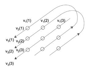
Figure A1. Circular convolution operation on two three-dimensional vectors  $v_1$  and  $v_2$ . Illustration adapted from Plate (1995).
