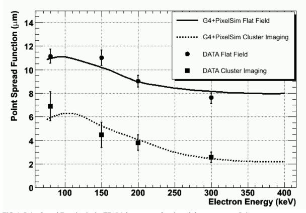
FIG. 1. Point Spread Function in the TEAM detector as a function of electron energy. Points represent measured values in "integrating" and "counting" imaging modes, and curves represent predictions from simulation.
