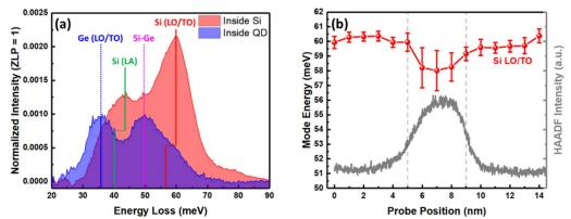
**Figure 2.** Phonon response of a single Si/Ge QD. (a) Background subtracted phonon signals. The red color denotes the signal in pure Si while the blue represents the signal when the probe is placed inside the Si/Ge QD. (b) A nanometer step line scan across a single QD, along with corresponding HAADF intensity.
