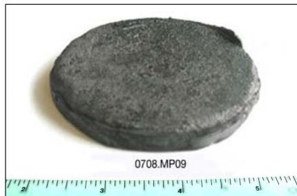
Figure 1. Typical carbon foam produced by the one-step process developed at Wright Materials Research Co. (WMR).
