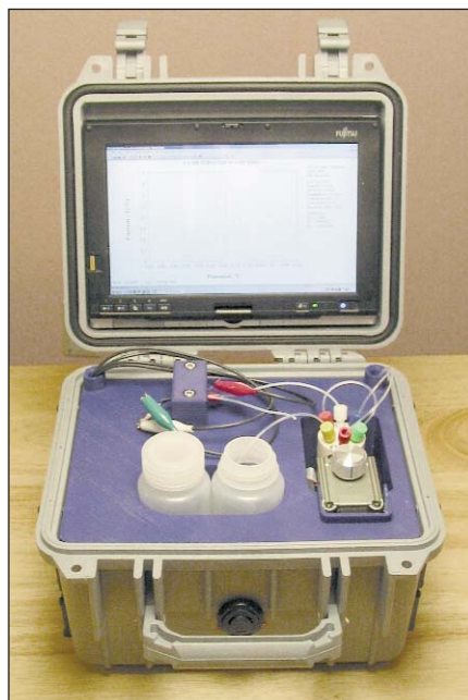
Figure 1. The biomonitoring detection system, developed by the Pacific Northwest National Laboratory, uses two classes of sensors to analyze water, saliva, or urine samples. The system is also being evaluated for use with blood samples. Although small and portable, the system provides detection levels at parts-per-billion.
