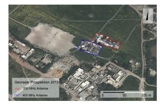
Figure 2. Results of the georadar survey, the upper part using deeper penetrating 200 Mhz antenna in the cavea area, the lower part 400 Mhz antenna in the arena area (M. Broisch).
