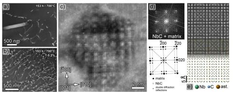
Figure 1. HAADF-STEM image of Sanicro 25 alloy (a) aged only and (b) aged & cyclically loaded with total strain amplitude of 0.2% at 700°C for 153 h. (c) NbC precipitate overlapping with matrix and forming Moiré-like contrast in HAADF-STEM [001] zone axis imaging. (d) FFT pattern & schematic corresponding to image (c). (e) Simulated Moiré-like contrast. HAADF-STEM image simulated along [001] zone axis is compared with structural model of overlapping NbC and austenitic matrix.
