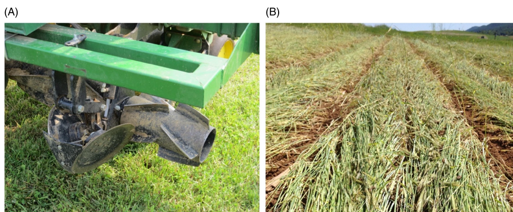
Figure 1. (A) Integrated roll-crimper and double-disk row-cleaning system mounted on planter toolbar (ZRX; Dawn Equipment, Sycamore, IL), which is designed to (B) part standing cover crop residue away from intrarow zone and roll-crimp toward interrow zone in a one-pass plant and roll-crimp operation.
