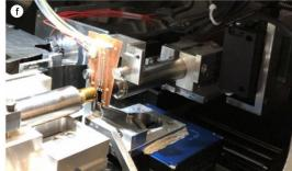
**Figure 1.** Microfluidic – based flow electrochemical cell for *in situ* and *operando* electrocatalysis studies [12]. (a-e) Details of the cell. The SiNx window area is 240 μm wide and 100 μm high. The active measurement area (dark circle on the WE) is 20 μm diameter, and has a ~10 nm Au thickness (plus 100 nm SiNx, and 2-3 nm Cr). (f) Photo of the cell inside the CLS ambient STXM.
