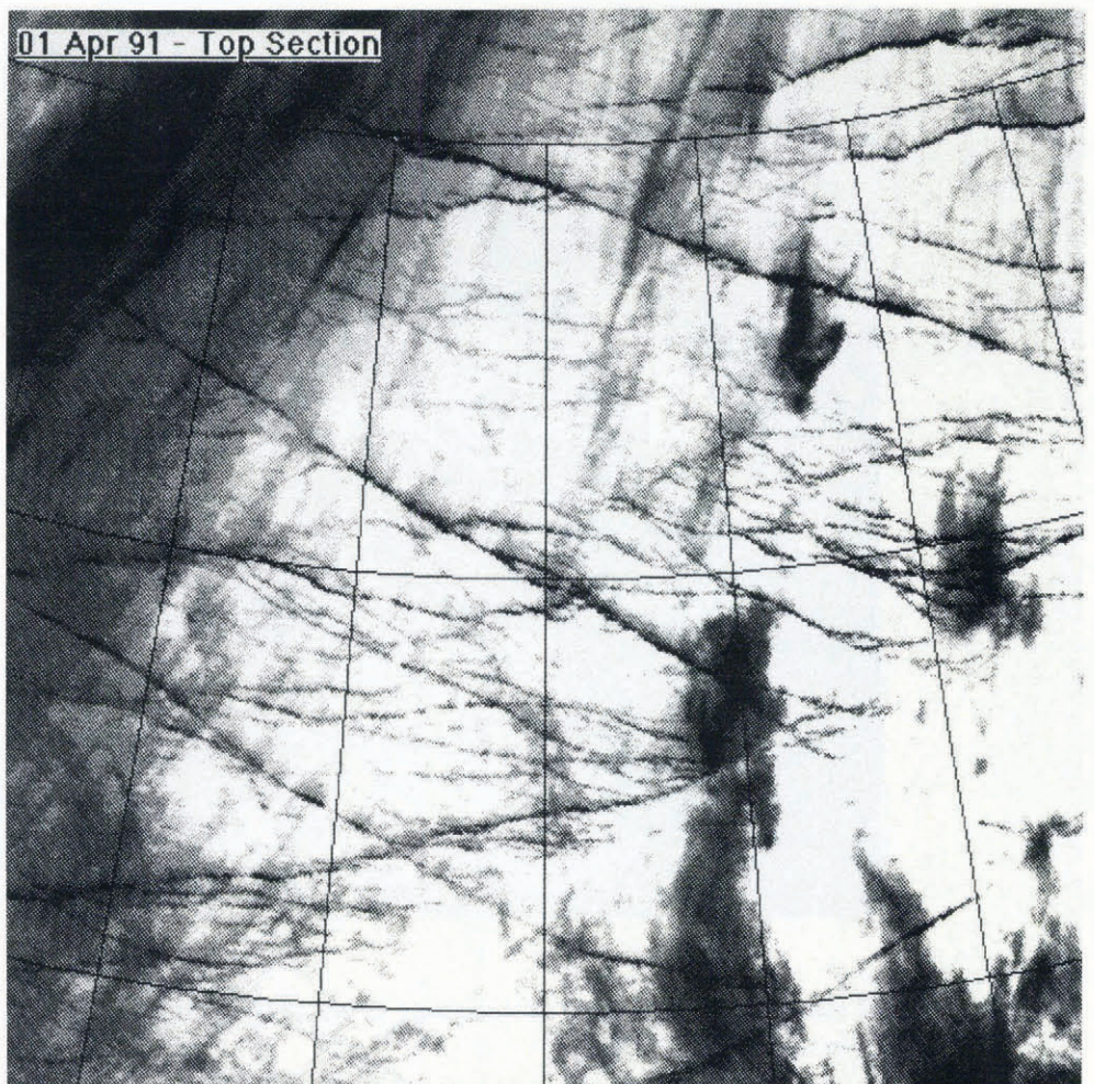
Fig. 8. AVHRR image (1 km resolution) for 1300 h GMT, 1 April 1991 showing that within the larger-scale ( \approx 150 km) lead features are smaller-scale ( \approx 10 – 20 km) lead structures of similar shape and with similar breaking angles ( \approx 30^\circ ).
