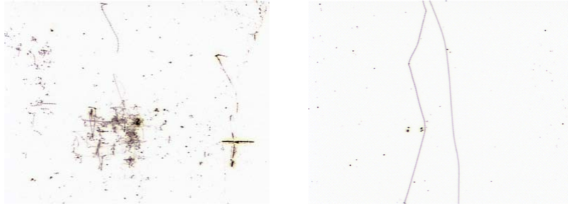
Figures 1 and 2: Scratches and debris found on a new microscope slide (field dimensions: 700\mu\text{m} \times 930\mu\text{m} ).
