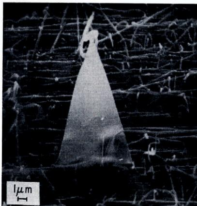
Fig. 5. Tape-like features in previously deformed ice.
