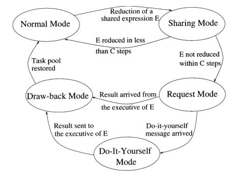
Fig. 5. A state-transition diagram of the CSM algorithm that handles do-it-yourself messages.
