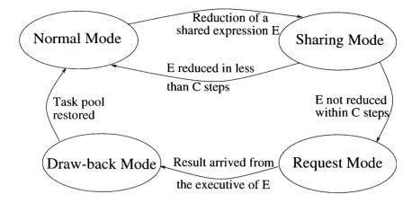
Fig. 2. A state-transition diagram describing the CSM algorithm.
