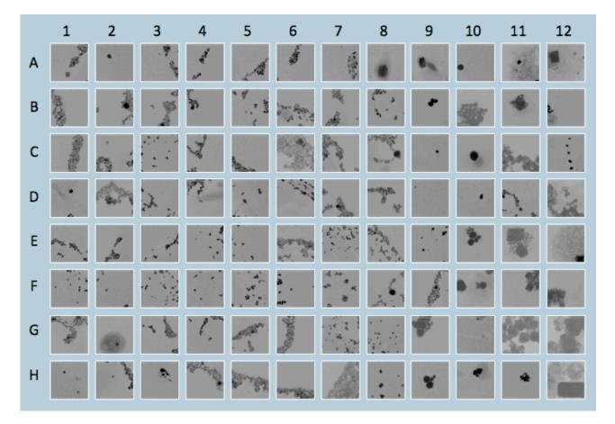
**Figure 2.** Thumbnail images (62,000x magnification) of 96 different samples from a single TEM grid; 10-20 images of each sample were obtained, which is sufficient to provide a statistically useful sample size.
