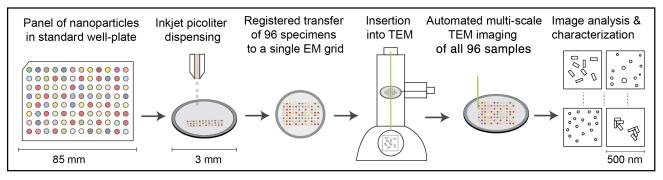
**Figure 1.** High-Throughput TEM Specimen Preparation Using Piezo-Based Picoliter Dispensing Inkjet transfer of multiple samples from well-plates to single EM grids followed by automated multi-scale TEM imaging. The goal is to increase the throughput of the imaging by 100x and reduce the sample volumes by 1000x.
