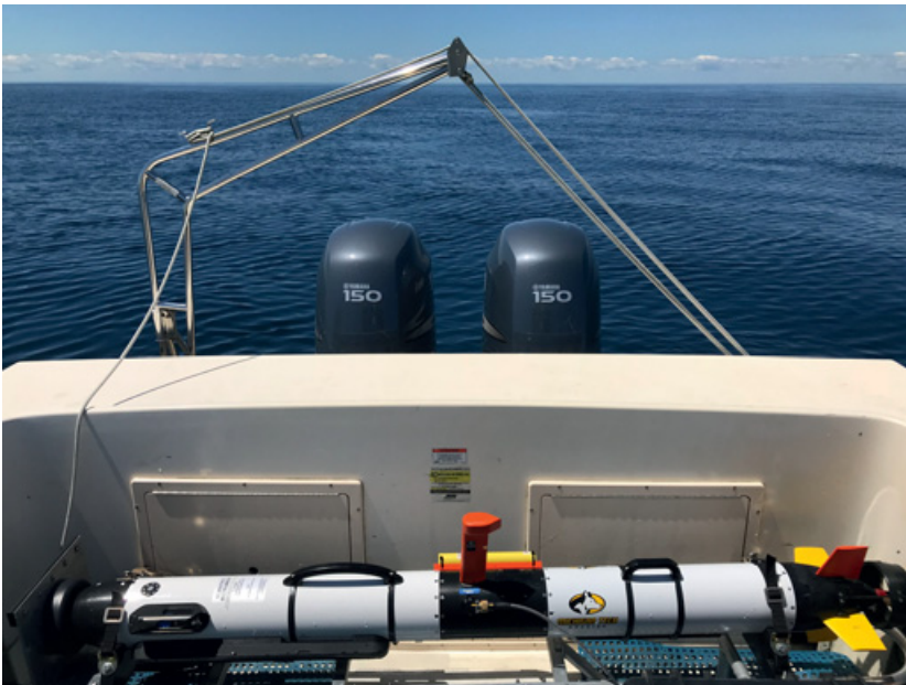
Figure 11 An autonomous underwater vehicle equipped with side-scan SONAR operated off a 7.6 m Parker, S/V Blue Traveler , Lake Huron, Great Lakes, USA.
