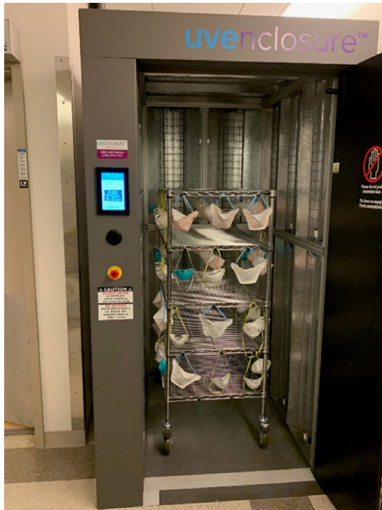
Fig. 1. Respirators are suspended from a wire shelving unit, then rolled into the ultraviolet (UV) machine for ultraviolet germicidal irradiation (UVGI).
