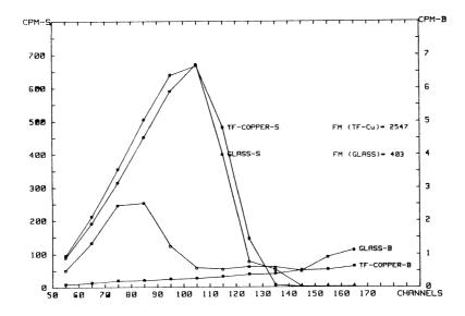
Fig 1. Radiocarbon (S) and background (B) spectra for glass and teflon vials
