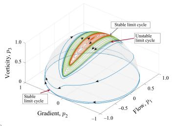
Figure 7. In  $R_{flow-vort}^{(1)}$  (shown here for c = 0.005,  $\kappa = 10$ , c De = 0.48), trajectories of particle orientation starting near the FGP (blue) spiral into the plane. Globally they emanate from an unstable limit cycle – the boundary between blue and green trajectories (that are started very close to each other in this numerical integration). There is a stable limit cycle above this unstable limit cycle at the boundary between green and orange trajectories.
