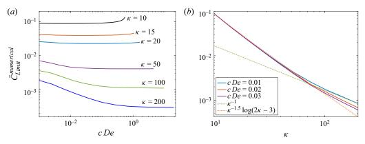
Figure 13. (a) The location of the stable limit cycle at different c De and  $\kappa$  at c = 0.005 (nearly identical curves are obtained for other polymer concentrations in the range  $0.01 \le c \le 0.2$ ) indicated by the average  $C = \sqrt{p_2^2 + p_1^2/\kappa^2}/p_3$ ,  $\bar{C}_{Limit}^{numerical}$  on the limit cycle. Here C = 0 is the vorticity axis and  $C = \infty$  is the FGP. (b) The  $\bar{C}_{Limit}^{numerical}$  on the limit cycle versus  $\kappa$  at low c De.
