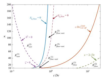
Figure 2. The  $\kappa$ -*c De* parameter space, for c = 0.005, divided into regions with different qualitative behaviour of a particle's orientation dynamics. Here  $b^2$  and  $\zeta$  are given in (5.4) and (5.12*a*,*b*), respectively;  $\lambda_{2,flow}^{0-}$  and  $\lambda_{2,flow}^{0-}$  are in (5.14). The procedure for numerically obtaining  $c De|_{cut-off}^{Limit}$  is described in § 5.4.1.
