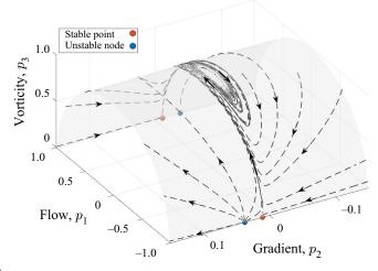
Figure 9. In  $R_{vort}^{(2)}$  (shown here for c = 0.005,  $\kappa = 50$ , cDe = 0.3), a particle's orientation trajectories approach the stable limit cycle around and near the vorticity axis. In contrast to  $R_{vort}^{(1)}$  (figure 6) where the trajectories spiral away from the FGP, here they leave the FGP monotonically. We show the region close to the flow–vorticity plane as this is where the different attractors lie. The grey surface is the unit sphere, i.e. the orientation space.
