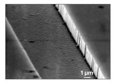
Figure 4. Scanning electron micrograph of inductively coupled plasma-etched ZnO. The features were patterned with photoresist that was removed prior to taking the micrograph. Image courtesy University of Florida.
