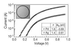
Figure 3. Current–voltage characteristics of Pd and Ag Schottky contacts on ZnO thin film deposited by pulsed laser deposition on r-plane (0112) sapphire substrate prepared at Leipzig University, Germany. The inset chart shows the ideality factors n and barrier heights  $\Phi_B$  of the two contacts in face-to-face configuration. An ideality factor of 1 indicates ideal diode behavior, with larger factors indicating deviations from ideality. The Schottky diode is shown in the inset.
