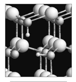
Figure 2. Atomic structure of a hydrogenated zinc vacancy in ZnO, based on first-principles calculations. Zinc atoms are the largest, oxygen atoms are medium-sized, and hydrogen atoms are the smallest. Image courtesy Xerox Palo Alto Research Center.
