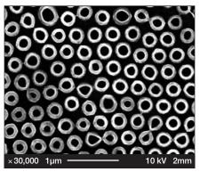
Figure 7. Scanning electron micrograph of ZnO "donuts" on a sapphire substrate generated using nanoporous polymer membranes (polymer template prepared by H. Xu, W. Goedel, M. Moeller). The diameter of these rings is ~300 nm and the wall thickness is ~100 nm. Image courtesy University of Ulm.
