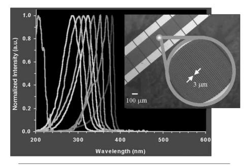
Figure 6. Visible-blind (transparent to visible light) UV detectors fabricated using compositionally tuned MgZnO thin-film alloys grown on a sapphire substrate. The graph shows the optical response in different regions of the linearly graded UV detector array, demonstrating the ability to tune the optical response. The inset image shows the linearly graded UV detector array. Courtesy of CSR, University of Maryland, and Blue Wave Semiconductors, Inc.
