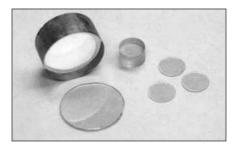
Figure 1. Melt-grown ZnO ingots and wafers. Courtesy Cermet, Inc.
