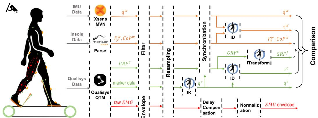
**Figure 2.** Data processing pipeline. The processing arrows in orange color are for the wearable measurement system. The processing arrows in green color are for the laboratory-based measurement system. The red arrows are the EMG processing steps.
