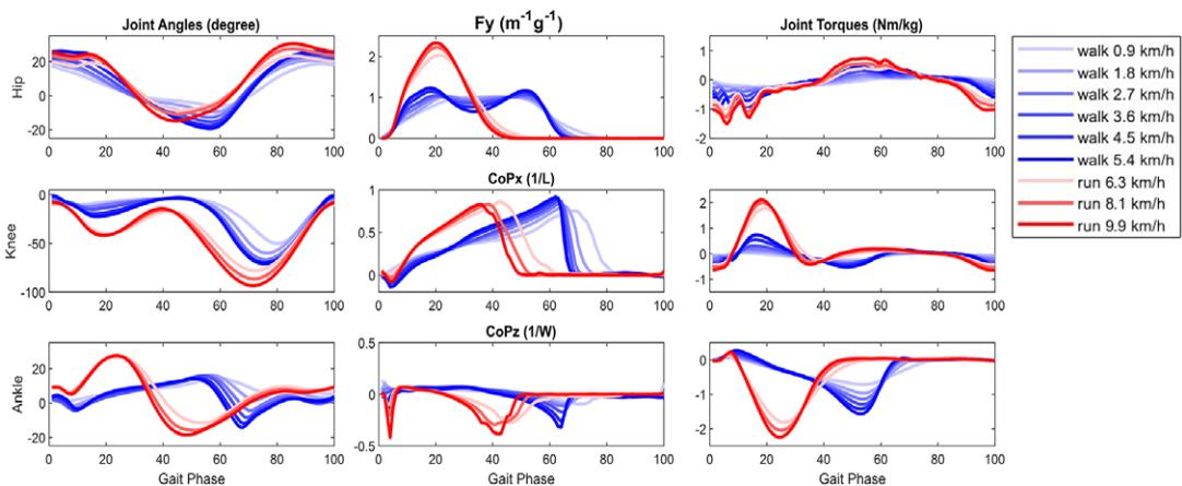
**Figure 8.** Averaged Joint angles, GRFs, and joint torques in the sagittal plane calculated from the wearable measurement system for all participants. The walking trials were plotted as the blue line with the shade indicating the speed. Correspondingly, the running trials were plotted in red.
