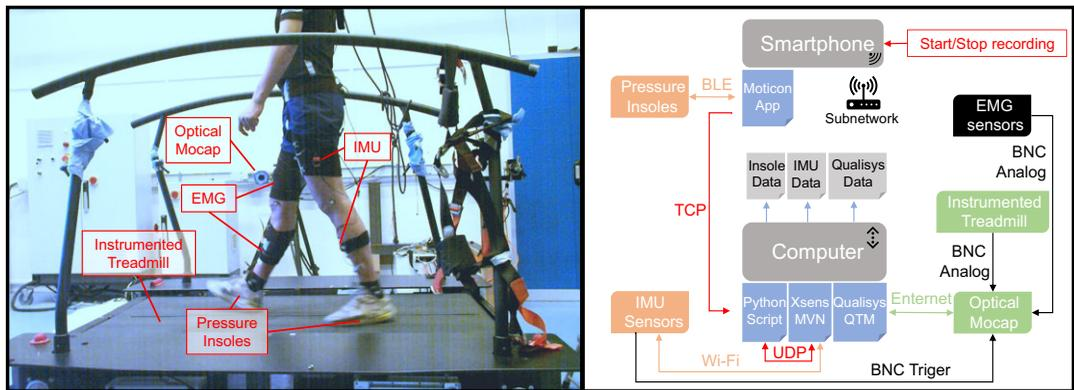
**Figure 1.** Experimental setup (left) and sensor hardware synchronization architecture (right). The pressure insoles and the IMU sensors (in orange color) form the wearable system. The optical mocap and the instrumented treadmill (in green color) form the laboratory-based system. EMG sensors were indicated with black color, since they can belong to either side.
