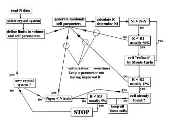
Figure 2. Flow diagram for McMaille.
