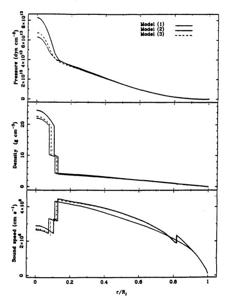
Fig. 39.1 Variation of the pressure, density and sound speed along the radius normalized to the Jovian radius, for the models of Chabrier et al. 1992.
