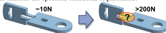
Figure 1. Snap-fit connection - The objective is to design a geometry with a holding force of more than 200 N that can be reused twice without damage
