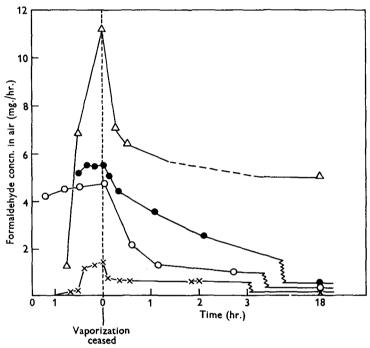
Fig. 6. Formaldehyde concentration in disinfectors A and B. The graphs are adjusted so that the times at which vaporization ceased coincide.  $\times$ , disinfector A with five or six mattresses, ambient temperature;  $\triangle$ , disinfector B with no mattresses, 40–45° C.;  $\bigcirc$ , disinfector B with one mattresses, ambient temperature.
