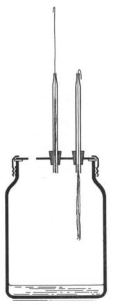
Fig. 3. Arrangement of jar disinfection experiments. During tests the threads hung free in the jar as shown on the right; they could be withdrawn into the glass tube (centre) and then the tube and rubber bung removed to enable samples to be taken.
