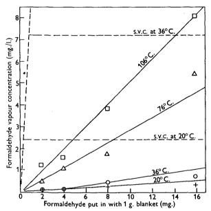
Fig. 7. Formaldehyde vapour concentrations in 125 ml. flasks containing various quantities of formaldehyde and 1 g. blanket at four temperatures. s.v.c. = saturated vapour concentration.
