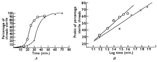
Fig. 4. Sterilization of heavily infected threads; formaldehyde 1.0 mg./l., at  $20^{\circ}$  C. and R.H. 58%. A, percentage of sterile threads plotted against time; B, probit of percentage of sterile threads plotted against log time.  $\bigcirc$  and  $\times = \text{results}$  of two separate experiments.
