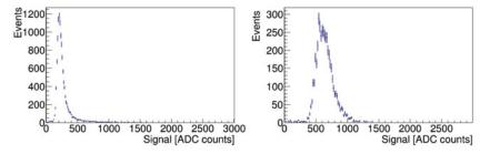
Figure 2. Energy loss within the Trigger System: on the left atmospheric muons; on the right 228 MeV protons acquired during a dedicated beam test.
