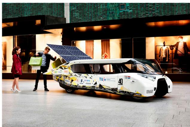
**Figure 4.** Solar family car 'Stella Lux', equipped with 5.8 m<sup>2</sup> of solar cells and a 15 kWh battery pack (Photo copyright Bart van Overbeeke; Courtesy: Solar Team Eindhoven).
