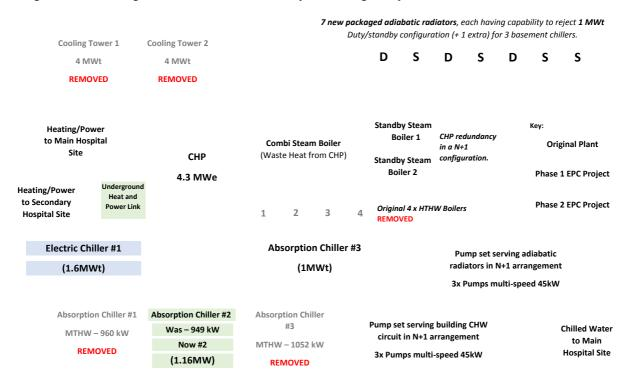
Figure 1. Modelling of the original and current hospital installations
