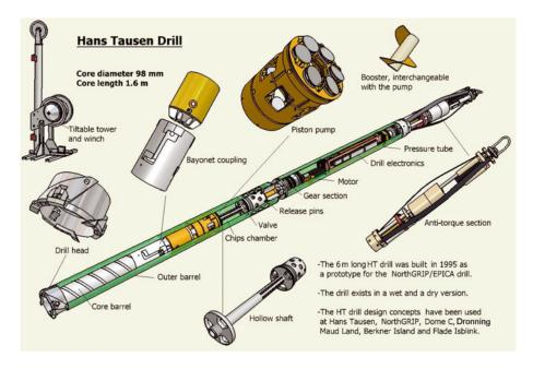
**Fig. 3.** The major components of the HT drill. The first version, a prototype for the deep NorthGRIP and EPICA drills, was tested on Hans Tausen Ice Cap in 1995; it did not have the pump or the bayonet coupling installed. See text for further explanation.
