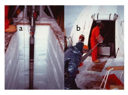
**Fig. 6.** Hans Tausen 1995 drill test. (a) The drill hangs in the drill pit from the shallow winch and tower unit. The base of the winch is seen at top, and the drill parts from top are anti-torque section, (short) motor section and top of chips chamber. (b) S.B.H and P.J. mount the core barrel and hollow shaft inside the drill. When this unit is pulled out, all the chips in the chips chamber will follow, with the top valve acting as piston. The rest of the drill is inside the white dome tent.
