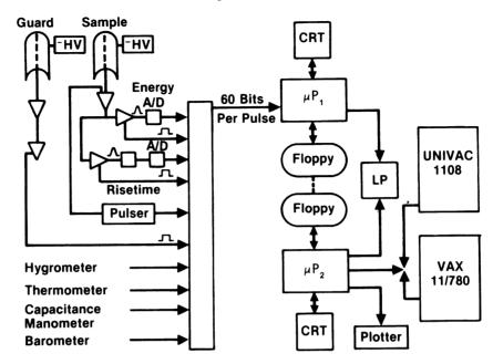
Fig 1. Structure of the microprocessor( $\mu P$ )-controlled data acquisition and processing systems. LP = Line Printer
