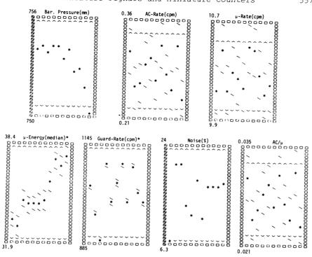
Fig 2. Multiparameter control chart (aerosol sample #561-562) showing parameters monitored on-line during 11-segment, 2200 min counting period. (\*) indicates  $\chi^2$  significant at 5% level. (\*) equals  $\pm$  Poisson- $\sigma$ ; ( $\updownarrow$ ) equals  $\pm$ 2s limits. (Imperfect run, selected to show drift and noise.)
