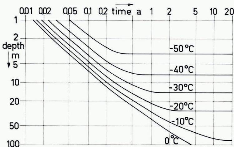
Fig. 3. Melting down of containers with 0.2 m radius and initially having 50 W with 1 year plus 50 W with 42 years mean life; from  $-50^\circ\text{C}$  to  $0^\circ\text{C}$  ambient firm temperature  $T + \Delta T$ .
