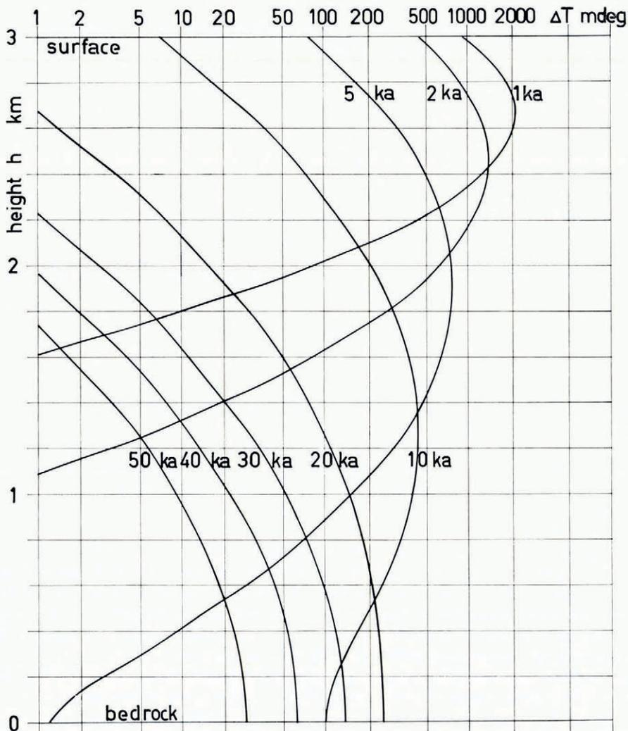
Fig. 2. Idealized profiles of the waste-induced temperature increase  $\Delta T$  from 1000 until 50000 years after dumping;  $A = 0.25$  m of ice/a.
