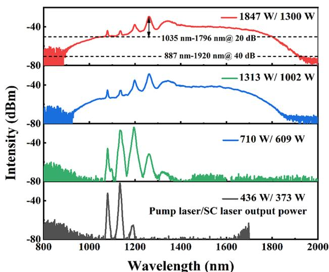
Figure 5. Output spectral evolution with pump laser power in the RFL with a half-open cavity.
