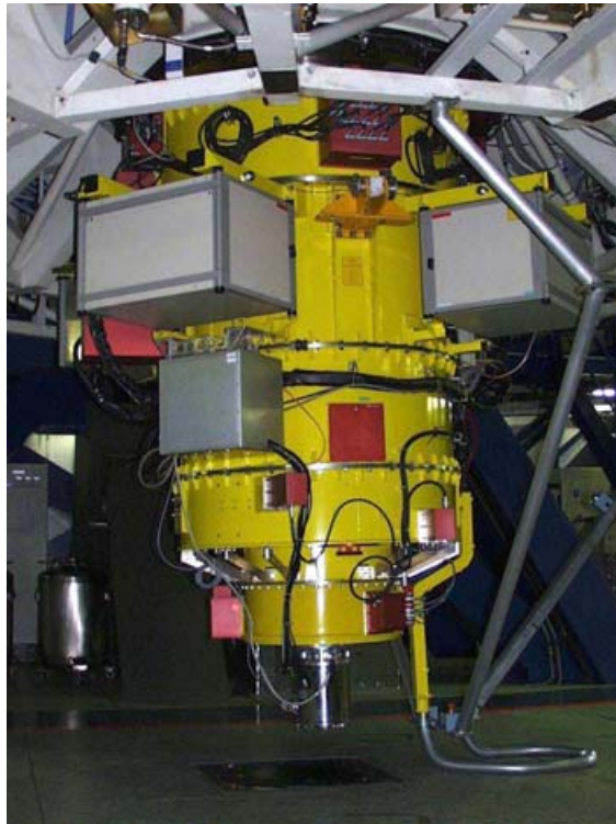
Figure 5. The FORS1 instrument of the VLT Unit 2 Kueyen permits one to obtain Stokes IQUV profiles in the optical range with a spectral resolution up to about 2000.
