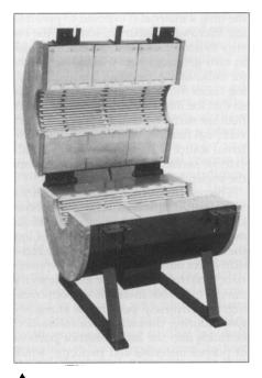
▲ Hinged Tube Lab Furnace: The M6018 single-zone hinged tube furnace from Lindberg/Blue M features graded insulation, reinforced hinges, and end vestibules for thermal uniformity and reduced heat losses. The furnace is rated at 5,600 W for operation on 240 V, 50/60 Hz, single phase; maximum operating temperature is 1100°C.
