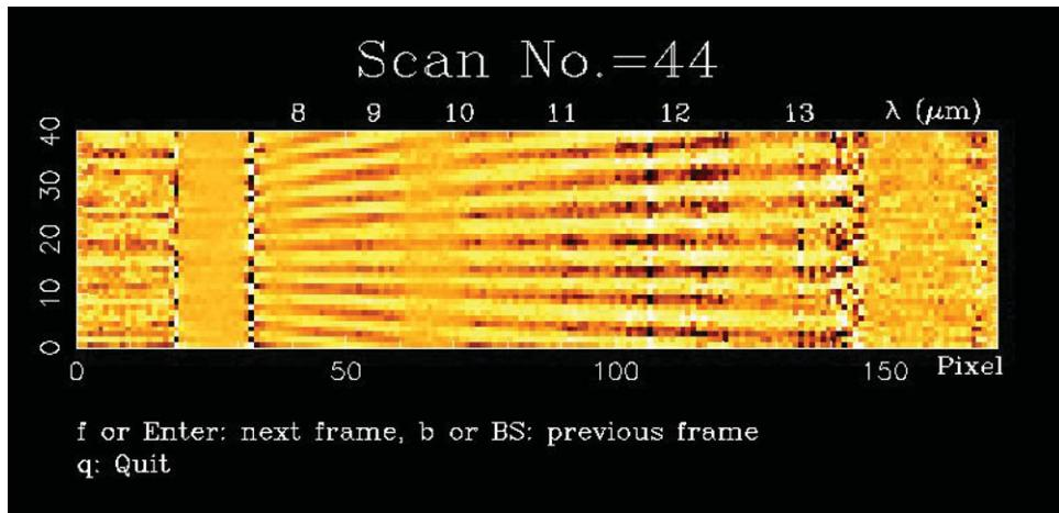
**Figure 2.** Spectrally dispersed fringes observed for WOH G64 with MIDI. These fringes were visualized by stacking 40 frames taken during one scan in the vertical direction. Each row corresponds to one frame.
