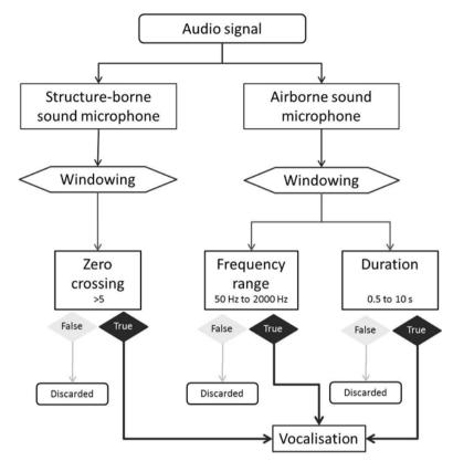
Figure 2 Process of call recording. Program flow chart of the developed algorithm for caller identification in dairy cattle (Bos taurus).
