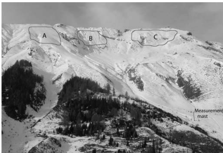
Fig. 1. Photograph of the Vallée de la Sionne test site showing the three possible release areas A–C and the 20 m high measurement mast. Photograph: F. Dufour.
