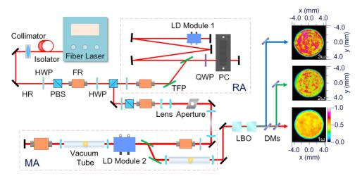
**Figure 1.** Schematic of the UV laser system and transverse beam profiles of the amplified pulses at  $1064 \text{ nm} (\omega)$ ,  $532 \text{ nm} (2\omega)$ , and  $355 \text{ nm} (3\omega)$  measured at their maximum energies via relay imaging. RA, regenerative amplifier; MA, main amplifier; HR, high reflector; HWP, half-wave plate; PBS, polarization beam splitter; FR, Faraday rotator; TFP, thin-film plate; QWP, quarter-wave plate; PC, Pockels cell; LD, laser diode; DM, dichroic mirror.
