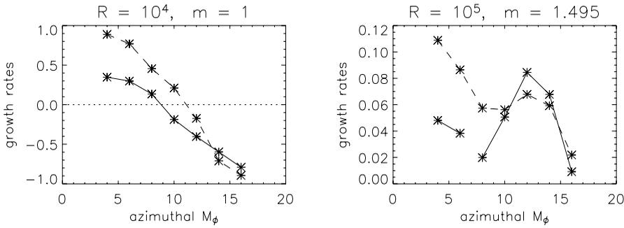
**Figure 1.** Linear mode growth rates obtained with two sets of parameter values. Results from the full magnetic field calculations are presented by the solid curve, while the averaged magnetic field is presented by the dashed curve. All modes show steady growth for  $R = 10^4$ . For  $R = 10^5$  the full calculation shows steady growth for  $M_\phi \leq 6$  and oscillatory growth for  $M_\phi \geq 8$ . All modes are oscillatory when the averaged magnetic field is used.
