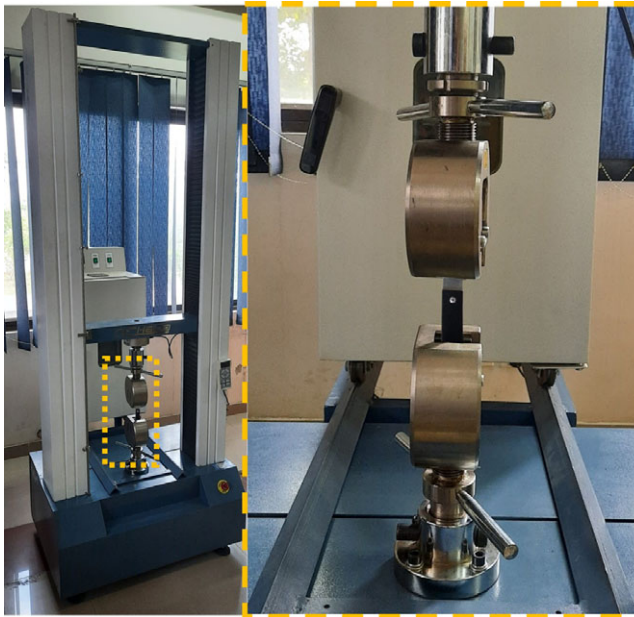
Figure 9. Experimental procedures for the tensile testing of the riveted joints.
