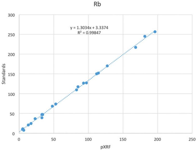
Figure 3. Comparison of pXRF and recommended values for rubidium (Rb) in 23 pressed powder geochemical reference standards. Values for goodness of fit ( $r^2$ ), slope and intercept are a measure of the performance of the Niton XL3t Ultra analyser and are used to derive calibration factors. Performance was good ( $r^2 > 0.9$ ) for all elements of interest.
