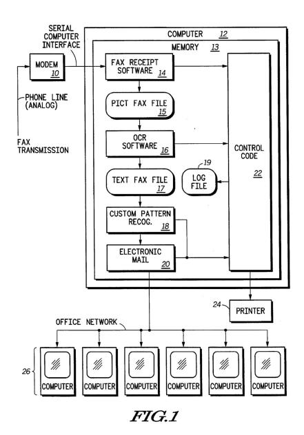
FIGURE 7.2 Block diagram of fax data processing system in accordance with the invention
