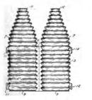
A bottle wrapper, comprising two similar parts, having corrugated sidewalls formed to surround a bottle, said walls being provided with integral fanges extending in wardly at one end of the wrapper to protect the corresponding end of the bottle, each of said parts being provided upon one edge with a pair of oppositely directed hook-like ears adapted to be interlocked for holding together the parts of the wrapper at one side, said parts being joined together at the opposite side.
