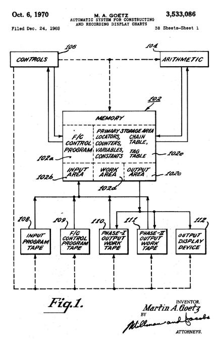
FIGURE 7.1 Schematic block diagram of a data processing system in accordance with the invention
