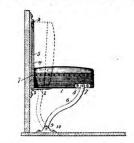
1. In a folding device of the character described, a seak, a pair of legs plvoted at their upper ends to the lower part of the seat near its forward edge, floor-brackets, plvotal connections between the floor-brackets and the lower end of the legs, upright guides at the rear of and above the horizontal plane of the seat, said plvotal connections being disposed in advance of the plane of said upright guides and means upon the seat for sildably engaging said guides.
