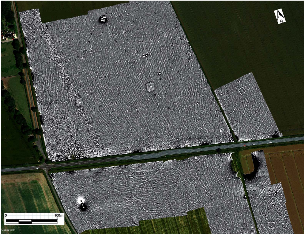
Figure 3. Magnetometer survey results. The frequent parallel lines across the plot are glacial features (figure by J. Lyall).
