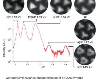
Cathodoluminescence characterization of a GaAs pyramid sample. The spectrum shows five main peaks corresponding to the five main structures in the pyramid. These are, from low to high energy: the quantum dot at the tip of the pyramid (QD), the vertical quantum wire (VQWR), the lateral quantum wires (QWR), the vertical quantum wells (VQW), and the quantum well along the sides of the pyramid (QW). SE is secondary electrons.
