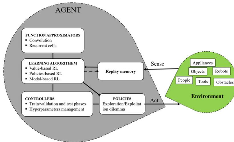
Fig. 10. General schematic of deep RL methods.<sup>172</sup>
