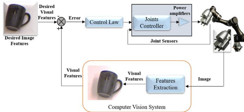
Fig. 7. Block diagram of direct visual servoing (adopted from ref. [1]).
