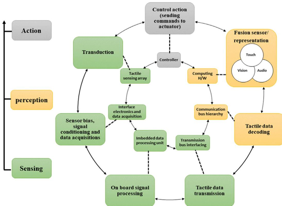
Fig. 5. Block diagrams of robotic tactile sensing system (adopted from ref. [76]).
