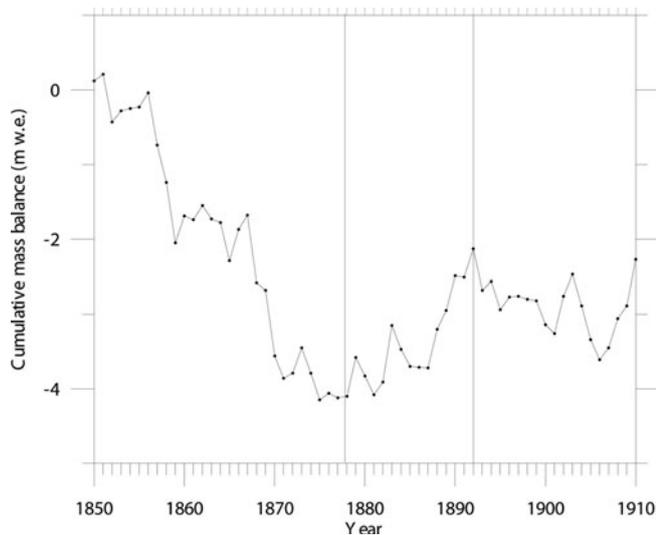
**Fig. 9.** Cumulative surface net balance (m w.e.) at the elevation of the former upper cavity (3165 m a.s.l.) between 1850 and 1910 from a reconstruction using homogenized precipitation and temperature data.
