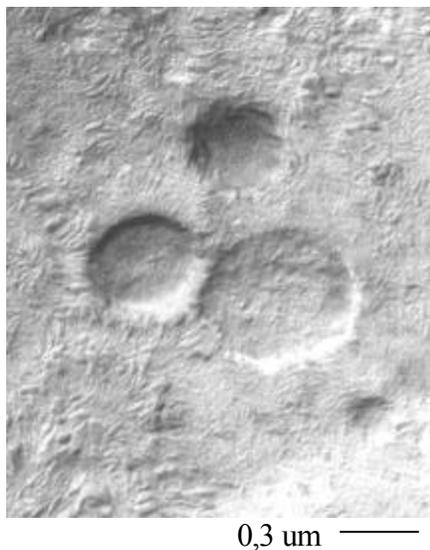
Figure 1. TEM permanganic etching followed by replication, LLDPE/iPP
