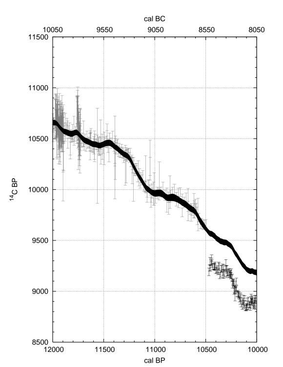
Figure A8 The Marine04 marine calibration curve (1-standard deviation envelope) and data with 1-standard deviation error bars increased by the laboratory error multipliers described in the text. The uncertainty in the calendar ages is not shown, but is taken into account in the random walk model.
