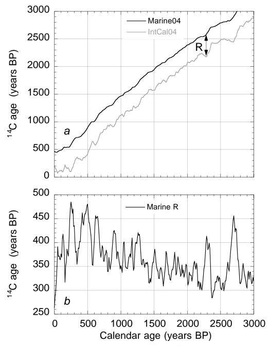
Figure 4 Global marine reservoir age "R" for the past 3000 yr. Atmospheric <sup>14</sup>C changes quickly following production spikes, but is muted in the ocean mixed layer. As a result, *R* calculated by the difference between IntCal04 and box diffusion model output (curve a) shows large variability (curve b). Beyond 10.5 cal kyr BP, when the Marine04 curve relies entirely on marine <sup>14</sup>C data sets, the global reservoir *R* is held constant at 405 yr (see Figure 2).
